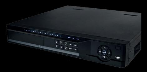
The FUSION-5X is a commercial 8 channel Penta-Tech DVR that combines 5 video technology formats. Especially selected for use with the S-COMM6 UVSS the FUSION 5X will support up to HD 1080p TVI image quality. The BNC inputs support all the major formats such as HDCVI, HDTVI, AHD and CVBS (Analogue). Four additional IP Cameras can also be added to the system to make a total of 12 channels.
