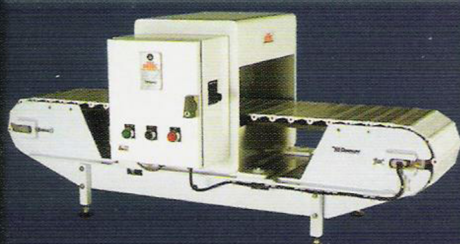
TSS CUSTOM DESIGNED CONVEYOR SYSTEMS INCORPORATING METAL DETECTOR UNITS
